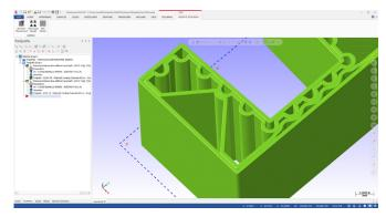
By incorporating the printing software within Mastercam, a single software can be used to create programs for both printing and subsequent trimming. If desired, this approach easily integrates with existing CAD/CAM systems for everything but the print programming function.
