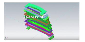
The 3D computer model, in an industry standard solid, surface or mesh file format, is loaded into Mastercam software and Thermwood's LSAM Print<sup>3D</sup> utility is used to create a print model and generate the CNC machine code needed to actually print the part.
