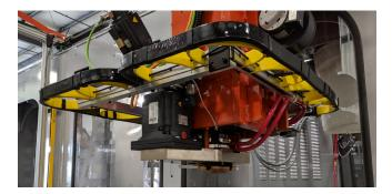
LSAM machines use a new, Thermwood developed, "MELT CORE" print head. Advantages of this design include much tighter control of print bead size, the ability to change bead dimensions while printing, the ability to print at high output rates without surging problems, better fusion between printed layers and a more void free printed structure. This unique print head design incorporates three servo drives, but unlike the servo drives that operate the machine, they are not programmable machine axes.
