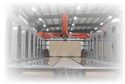
LSAM is intended for serious industrial production. It is not a lab, evaluation or demonstration machine, but is instead a full-fledged industrial additive manufacturing system intended for the production of large scale components.
