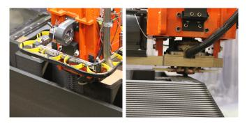
Since it tends to squeeze out air that might otherwise be trapped between layers, this compression wheel results in superior bonding between printed layers and a better, void free structure. Thermwood's additive print head housing can accommodate interchangeable melt cores. A melt core consists of a feed housing, extruder and polymer melt pump and determines just how fast material can be printed.
