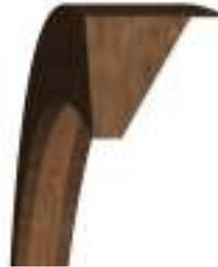
The last pair of images shows the tool path still starting at the bottom right with a -4" plunge, but this time a 2" left offset is used. Notice again that the direction the cut moved on the part by changing the offset, this time from the top toward the bottom. Why did it move in the opposite direction? Because the tool path started at the opposite end of the part.
