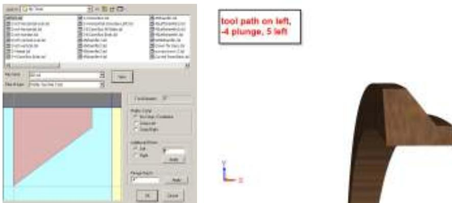
In the third pair of images, the tool path starts at the bottom right and has a -4" plunge with a 1" left offset.
