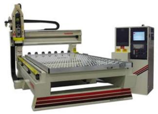
Thermwood fixed table machines have separate servo drives for each side of the gantry to prevent skewing and provide independent compensation for each lead screw, assuring squareness and accuracy.
