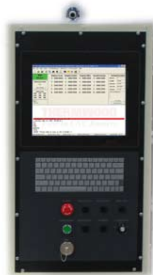
The nesting, CAM work and Post Processor are all in the control and are all automatic.
