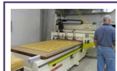
Using Automatic Load and Unload a single operator can run more than one upholstered frame system.
