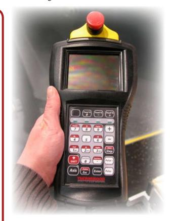
The Thermwood Hand Held Programmer is the single most powerful tool available for creating, modifying, editing and refining CNC programs at the machine. The Hand Held Programmer provides a vital link between the CAD/CAM programmer and the CNC machine tool.
