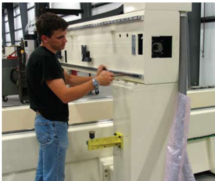
Eric Gehlhausen adjusting rail alignment
