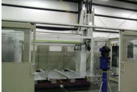
Large 5-axis machine being readied for volumetric compensation
