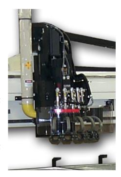
The Typewriter Style Automatic Tool Changer is equipped with five tool holder arms which are mounted in an arc in front of the spindle. The cutting tools used with this option are limited to 2" maximum diameter and 3" maximum length. This option comes with five tapered tool holders and five collets, and a preset tool holder fixture for changing cutter bits away from the machine. Additional tool holders and collets may be purchased from Thermwood.
