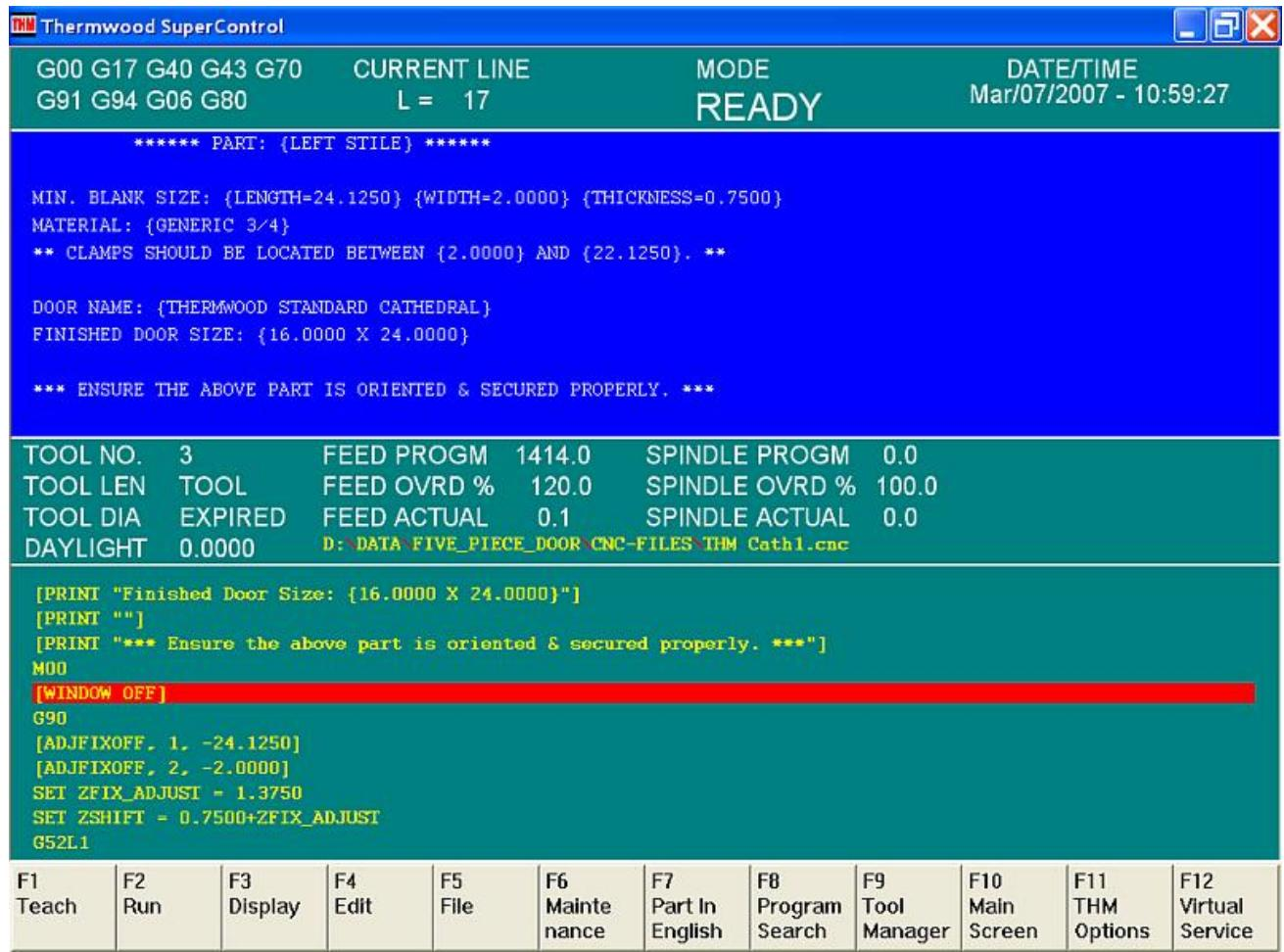
After the first part has run, you will then see additional information in the blue area of the SuperControl menu, alerting you that the next part is ready to be run.
