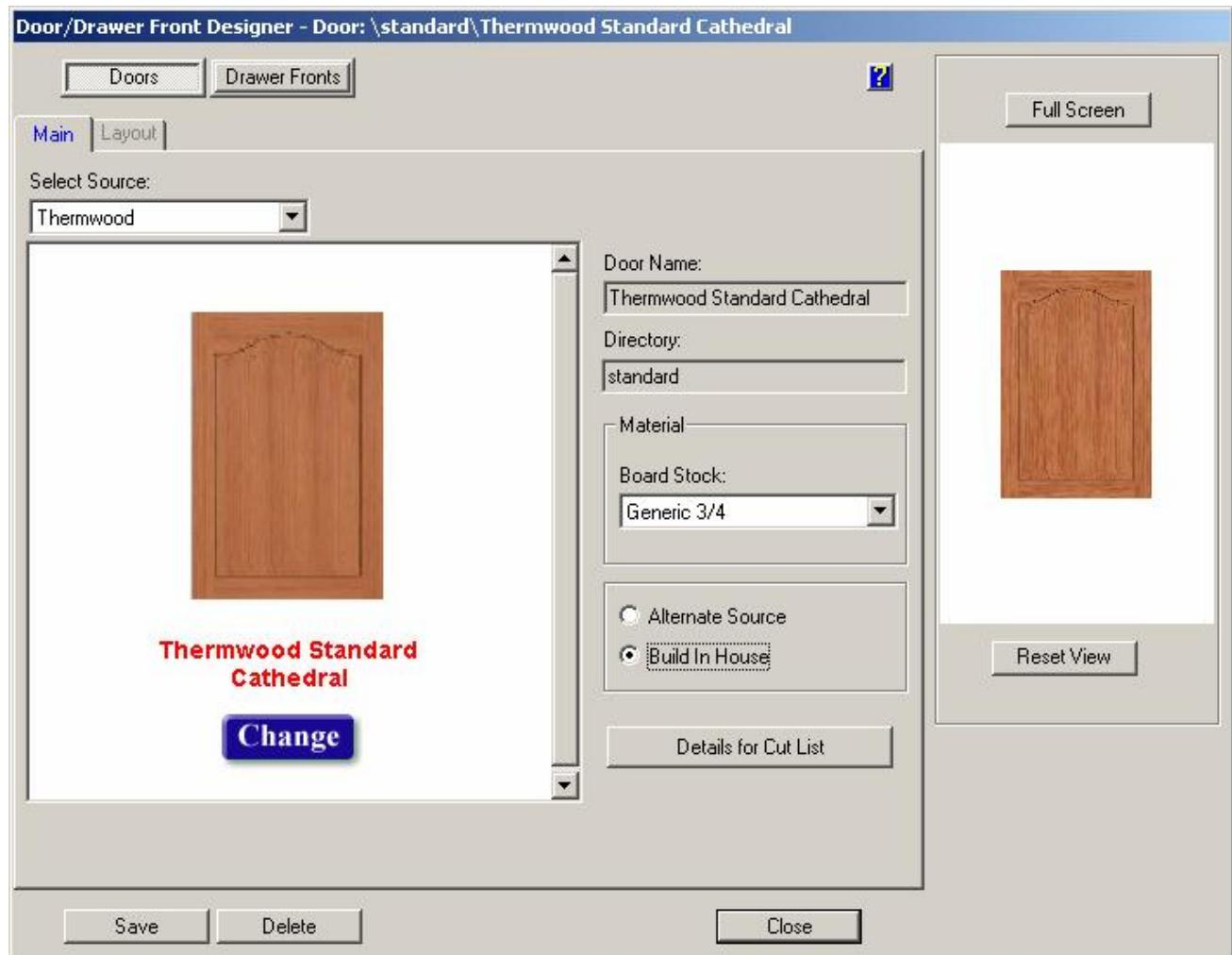
**NOTE:** When using the "Build In House" option for vendor door/drawer fronts, it is important to understand that what is displayed is just for reference. What you see graphically, and the settings that are displayed here and in the "[Sizing Details for Cut List](#)" area, may not correspond. The vendor door/drawer fronts will display with the rail and style widths and the material color/textures that are predetermined by the vendor's specifications.
