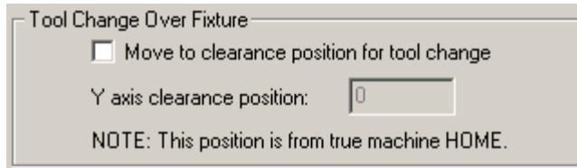
*NOTE: This feature ensures that there is no collision between any part of your work or fixture while the tool change operation is occurring. Also note that this clearance position is referenced from your Thermwood's Machine Home position!*
