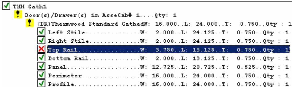
The checkboxes are used to deselect specific parts from the job. Green checks indicate that all parts are selected and will be processed. Clicking on (for example, one of the rails or stiles), will cause a yellow exclamation point marker to show in the Cabinet and Door Type selection area, alerting you that this job will proceed, but will not be complete. Clicking anywhere above the component list will cause a red "X" to be displayed, showing that this job will not be processed.
