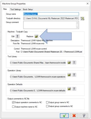
5.) On the *Open Machine Definition File* dialog, select the *Thermwood LSAM.mcam-rmd* file and then select *Open*. (Note: If using Mastercam Mill, select the file *Thermwood LSAM.mcam-mmd*)
