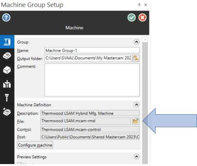
5.) On the *Open Machine Definition File* dialog, select the *Thermwood LSAM.mcam-rmd* file and then select *Open*. (Note: If using Mastercam Mill, select the file *Thermwood LSAM.mcam-mmd*)
