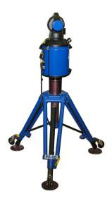
Volumetric Compensation, standard on all Thermwood CNC routers, dramatically improves the accuracy and quality of the machine. This state-of-the-art advanced technology, developed by Thermwood, is especially essential for large envelope five-axis machines. In this process, the laser measures the exact positions of the cutting head, in three dimensions within the working envelope, and compensates for any remaining error. The com-
