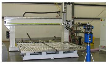
pensation then becomes integral within the machine's control providing precise positioning of the cutting head.
