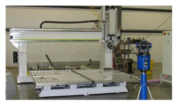
pensation then becomes integral within the machine's control providing precise positioning of the cutting head.
