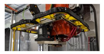
LSAM machines use a new, Thermwood developed, "MELT CORE" print head. Advantages of this design include much tighter control of print bead size, the ability to change bead dimensions while printing, the ability to print at high output rates without surging problems, better fusion between printed layers and a more void free printed structure.
