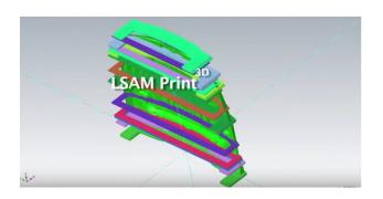
The 3D computer model, in an industry standard solid, surface or mesh file format, is loaded into Mastercam software and Thermwood's LSAM Print<sup>3D</sup> utility is used to create a print model and generate the CNC machine code needed to actually print the part.
