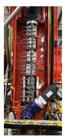
Thermwood's additive print head housing can accommodate interchangeable melt cores. A melt core consists of a feed housing, extruder and polymer melt pump and determines just how fast material can be printed.
