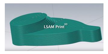
The process starts with a 3D computer model of the part. This design, in an industry standard solid, surface or mesh file format, is loaded into Mastercam software. Thermwood's LSAM Print<sup>3D</sup> software utility, which operates within Mastercam, is used to generate the CNC print program needed to
