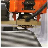
Since it tends to squeeze out air that might otherwise be trapped between layers, this compression wheel results in superior bonding between printed layers and a better, void free structure.
