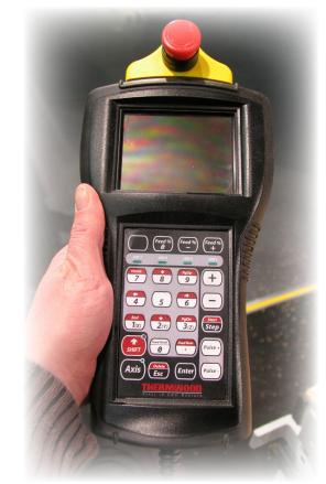
The Thermwood Hand Held Programmer is the single most powerful tool available for creating, modifying, editing and refining CNC programs at the machine. The Hand Held Programmer provides a vital link between the CAD/CAM programmer and the CNC machine tool.
