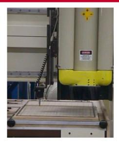
later in the program uses it. It can measure in either X, Y or Z-axes. The option comes mounted on an air slide, which mounts on one of the piggyback positions. In order to properly utilize this option the user must make use of the Thermwood Advanced Function Language programming. To program in AFL the person must be an experienced computer programmer.
