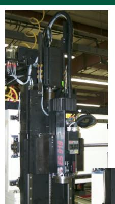
The Trackway Z Axis assembly is available on Model 40,42 and 53 machines. This option replaces the Z axis slide which was standard on these machines.
