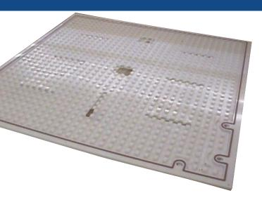
The Vacuum Plenum is available on most Thermwood machines. The Vacuum Plenum is made of half inch polyethylene and machined to fit the table top including mounting holds. These are grided tops that are covered with a sheet of spoilboard to assist in part hold down using vacuum.
