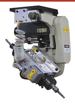
**7.5 HP Standard:** This Dual End Spindle has a collet chuck on each end of the spindle. Each has the capacity of holding a cutter with a maximum of a 1/2" shank and a maximum length of 3" extending from the face of the covernut. The cutter diameter should not exceed the diameter of the shank. The primary cutter is right handed and the secondary is a left handed cutter. Includes one 1/4", one 3/8" and one 1/2" collet.
