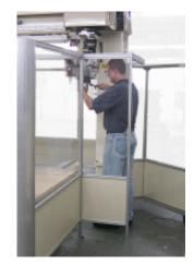
On a dual table machine it is possible to load and unload parts while the machine is in operation. Dual table machines have a center partition to separate the operator from the active table, where the trimming operation is occurring, while he is loading the non active table. The machine will stop if the head travels past the coordinates of the active table. If the tables are joined for a larger machining area, by removing the center partition, both doors have to be closed in order for the ma-
